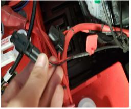
b. Disconnect the two green marked cables and remove the plug from the red connector. Plug the green connector into the red connector.
