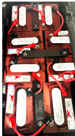
Figure 1. Beyond 4 Passenger with a total of 6 lead acid batteries. Batteries are located in the 2nd row storage, underneath the flip seat.
